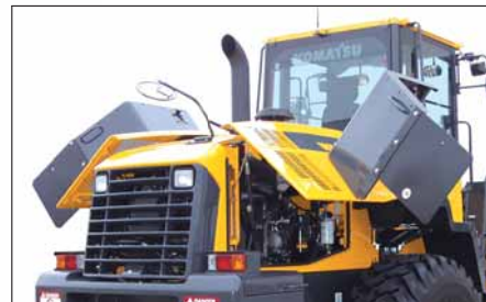
Gull-wing side doors lower locked position
